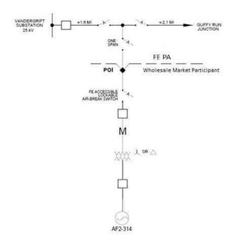
→ POI (POINT OF INTERCONNECTION) LOCATED AT FE PA OWNED SUBSTATION DEAD-END STRUCTURE WHERE CUSTOMER'S TRANSMISSION LINE TERMINATES
