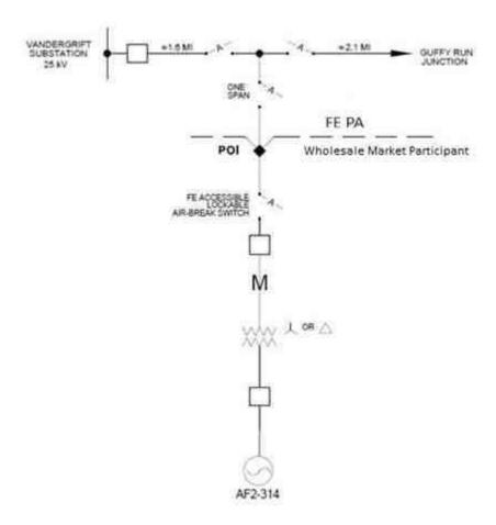
→ POI (POINT OF INTERCONNIECTION) LOCATED AT FE PA OWNED SUBSTATION DEAD-END STRUCTURE WHERE CUSTOMER'S TRANSMISSION LINE TERMINATES
