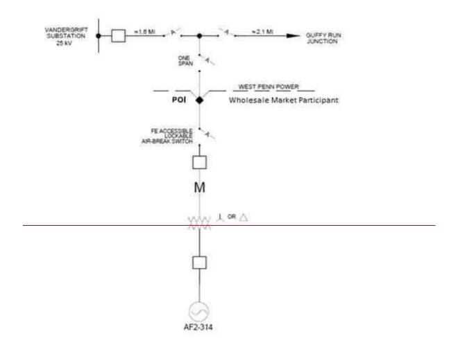
POI (POINT OF INTERCONNECTION) LOCATED AT WEST PENN POWER OWNED SUBSTATION DEAD-END STRUCTURE WHERE CUSTOMER'S TRANSMISSION LINE TERMINATES
