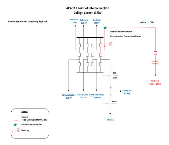
The Point of Interconnection ("POI") is at the first (dead-end) structure north of the College Corner 138 kV station fence. AEP owns the span from the College Corner 138kV station to the dead-end, including the jumpers and structure at the dead-end. Angelina Solar I, LLC owns the span connecting to the POI, and the 138kV generator lead line and remaining structures back to the AC2-111 generation collector station.
