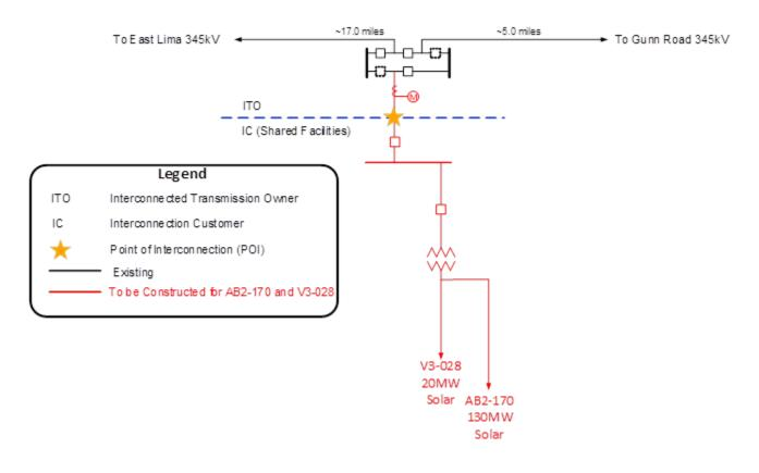
The Point of Interconnection is the first structure outside of AEP's Hardin Switchyard (such structure being located in Interconnection Customer's 34.5-345 kV Collector Substation) with the Interconnected Transmission Owner owning the first span of conductors including the optical (fiber) ground wire out of its station, and the Interconnection Customer owning the first structure.
