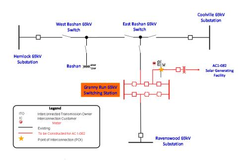
The Point of Interconnection is the first structure outside of the proposed Granny Run 69 kV station (such structure being located in Interconnection Customer's 34.5-69 kV Collector Substation) with the Interconnected Transmission Owner owning the span of conductors, and the Interconnection Customer owning the structure.
