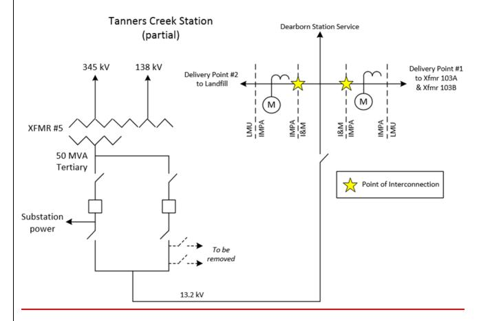
The Delivery Point #1 Point of Interconnection is at LMU's primary metering pole on LMU's retail customer's property with I&M owning the conductors up to LMU's primary metering pole.
