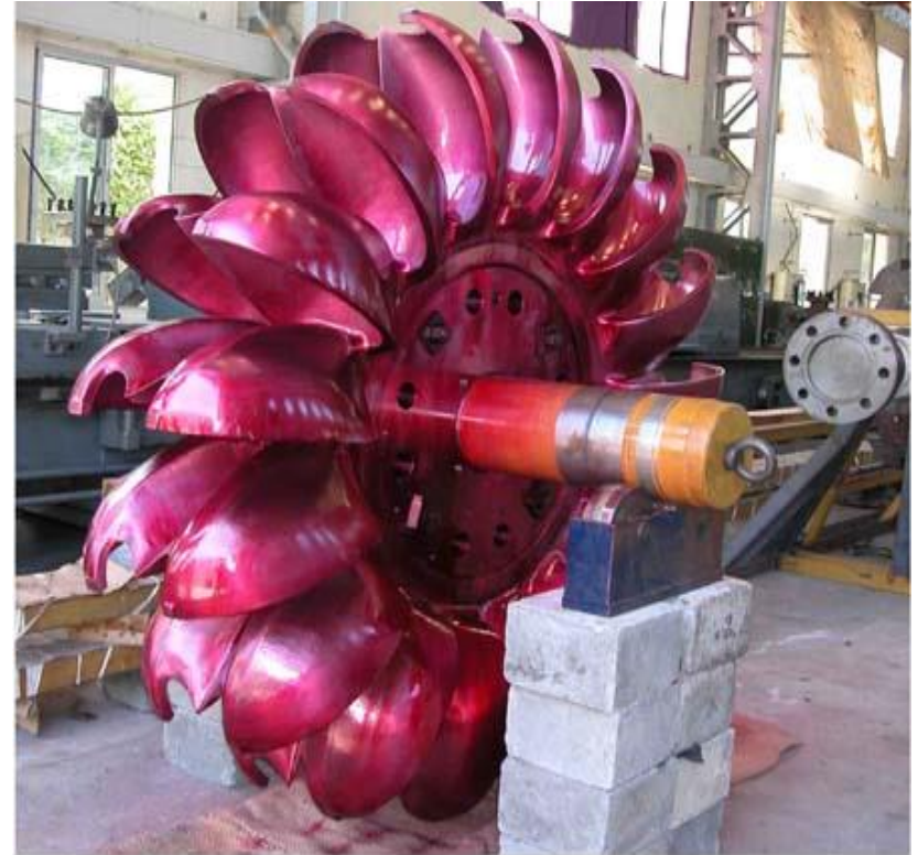
Repair & Refurbishment of Pelton Wheel Runner - DP Test
