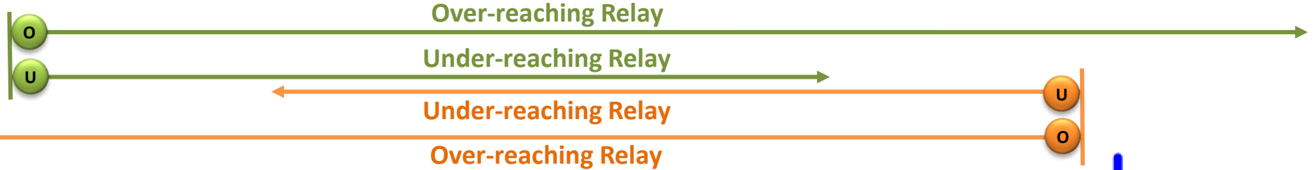
Permissive Under-Reaching Transfer Trip
