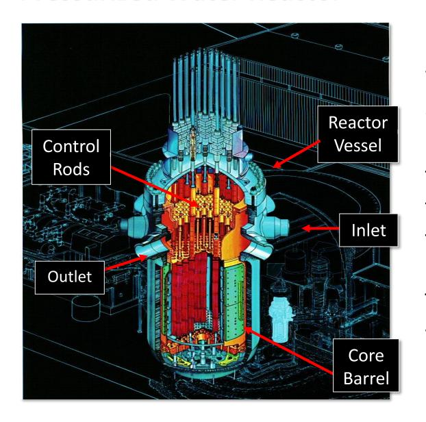
Water flows downward on the outside of the core barrel to the bottom of the reactor. The flow then turns upward in between the fuel rods from the bottom to the top of the reactor
