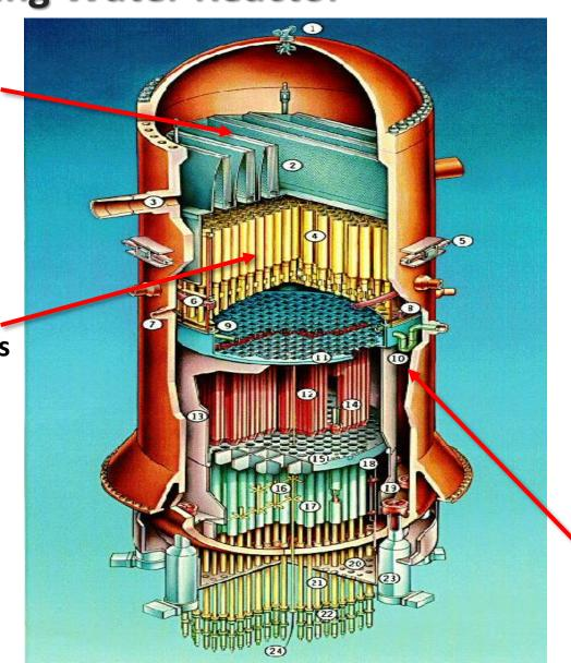
Water flows downward on the outside of the core barrel to the bottom of the reactor. The flow then turns upward in between the fuel rods from the bottom to the top of the reactor
