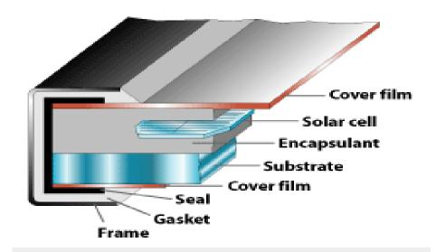
One typical flat-plate module design uses a substrate of metal, glass, or plastic to provide structural support in the back; an encapsulant material to protect the cells; and a transparent cover of plastic or glass.
