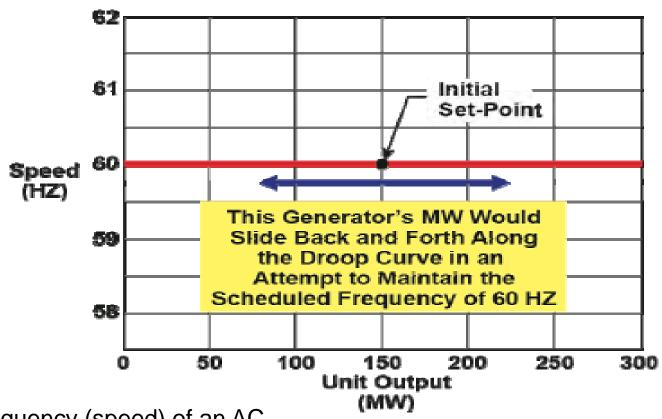
Controls the frequency (speed) of an AC generator
