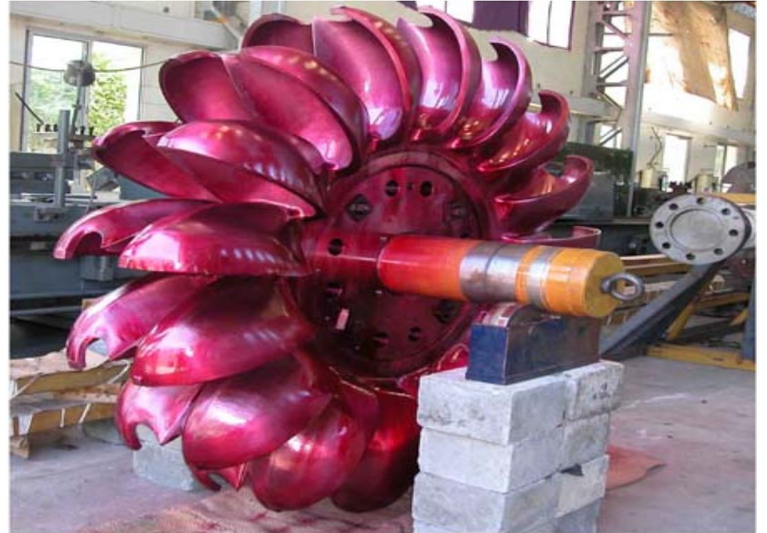
Repair & Refurbishment of Pelton Wheel Runner - DP Test
