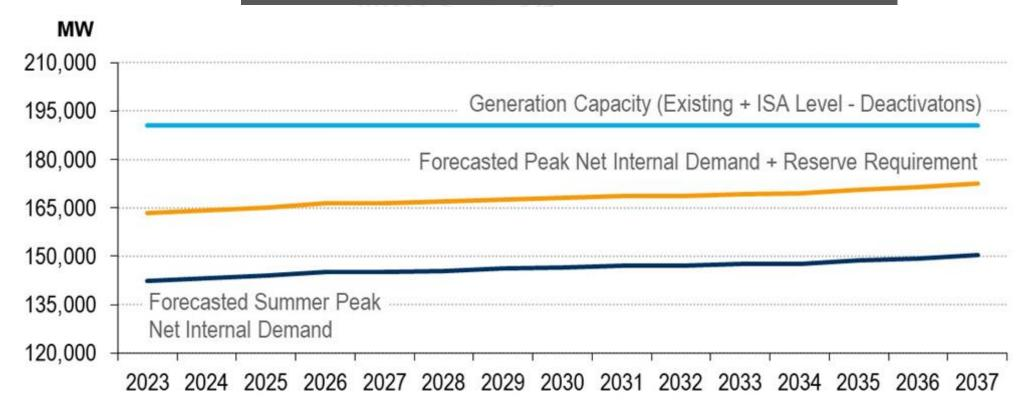
**Notes**: Generation includes existing and projected PJM internal capacity resources. Solar and wind resource capacity at 38% and 13% of maximum capability, respectively. Model informed by the 2027 RTEP Powerflow and the Generation Interconnection Queue.
