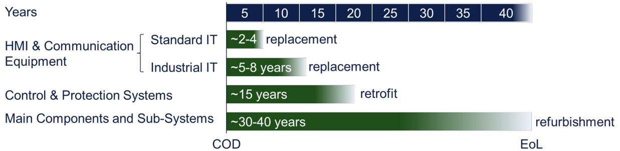
Figure 5-2 Illustration of Timing of Major O&M Activities for Converter Stations
