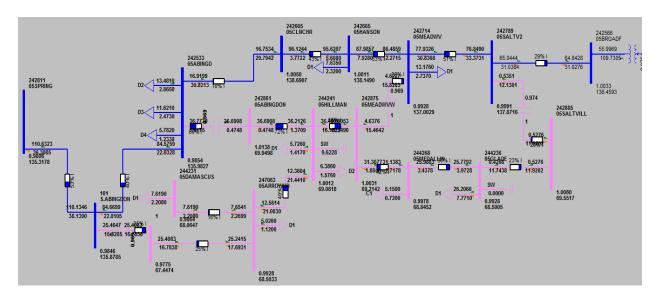
Figure D2: Loading on Abingdon – Hillman Highway 69 kV Ckt 1 for the loss of Broadford – Sulivan 500 kV Ckt 1 under this project
