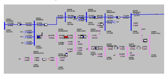
Figure D1: Loadabing on Abingdon – Hillman Hwy 69 kV Ckt 1 for the loss of Broadford – Sullivan 500 kV Ckt 1
