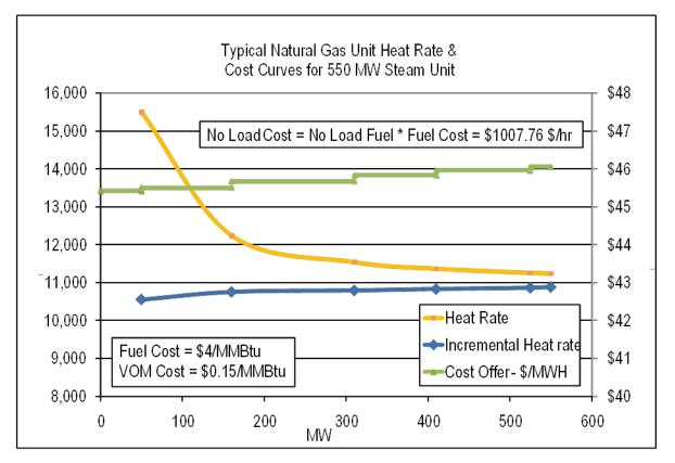
To avoid making adjustments to the No-Load Cost, first calculate the unit's Incremental Cost (\$/ MWh) at various outputs using the derivative of the Heat Input Curve:
