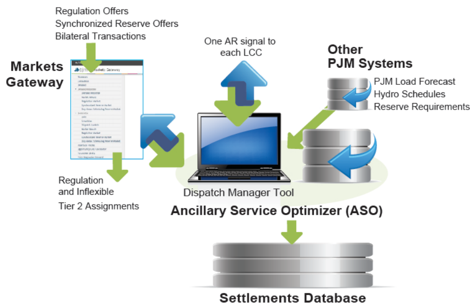
Exhibit 8: Synchronized Reserve and Regulation Data Flow
