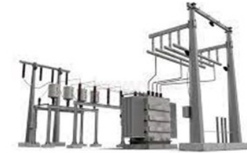
Substation B Limiting Element MVA Rating: 350 MVA Peak Loading in N-1: 125 MVA
