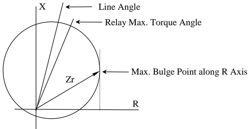
**Figure F-2 Lens Relay Characteristic showing Maximum Bulge Point**
