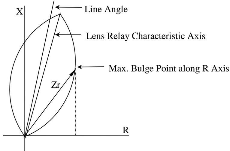
**Figure F-3 Straight Line / Blinder Relay Characteristic showing Maximum Bulge Point**
