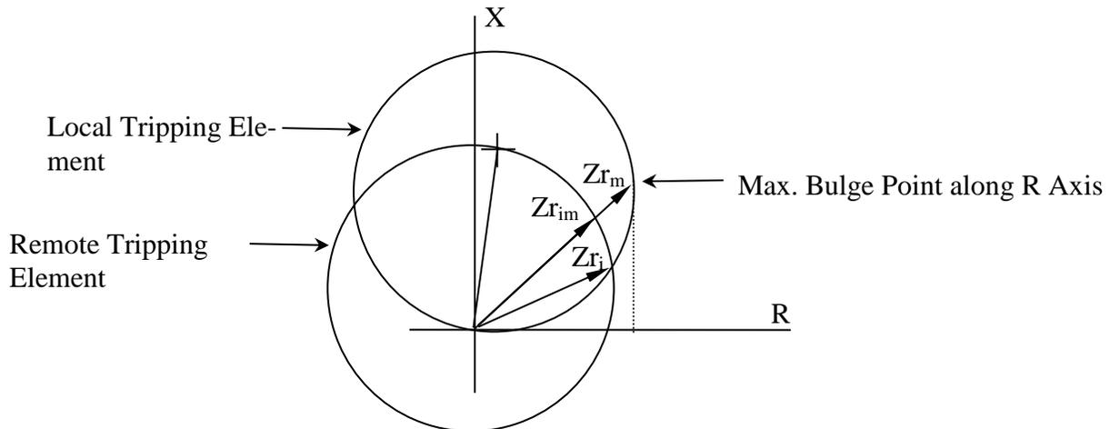
In rare cases, the maximum bulge point of the local tripping characteristic will fall within the tripping characteristic at the remote end of the line (See Figure F-7B). In these cases, the maximum bulge point of the phase tripping element should be used to calculate the DRTLL. Again, since the pilot scheme is a high speed-tripping scheme, a  $K_t$  corresponding to 0.53 should be used.
