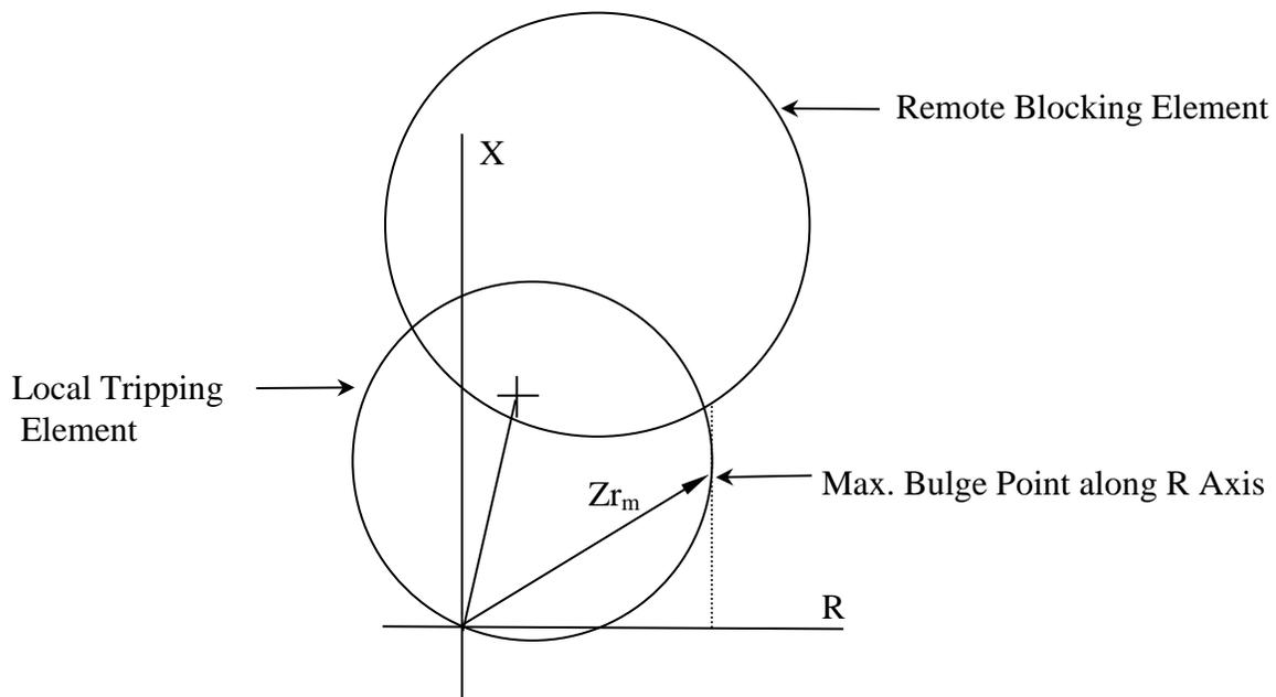
In rare cases, the maximum bulge point of the local tripping characteristic will fall within the blocking characteristic at the remote end of the line (See Figure F-6B). In these cases, a slightly higher loading limit can be realized by using the intersection of the tripping and blocking characteristic  $Z_{r_i}$  to calculate the DRTLL. Again, since the blocking scheme is a high speed-tripping scheme, a  $K_t$  corresponding to 0.53 should be used.
