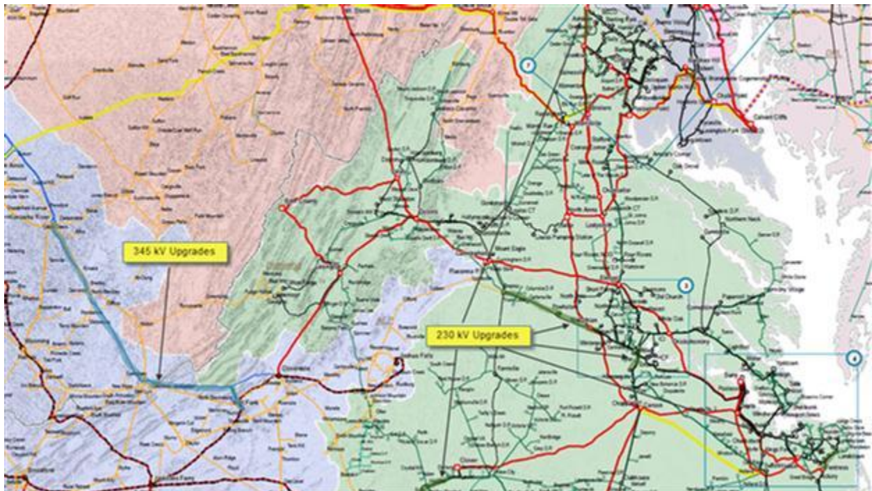
Figure 1-33: 30% LOBO Transmission Overlay – Dominion
