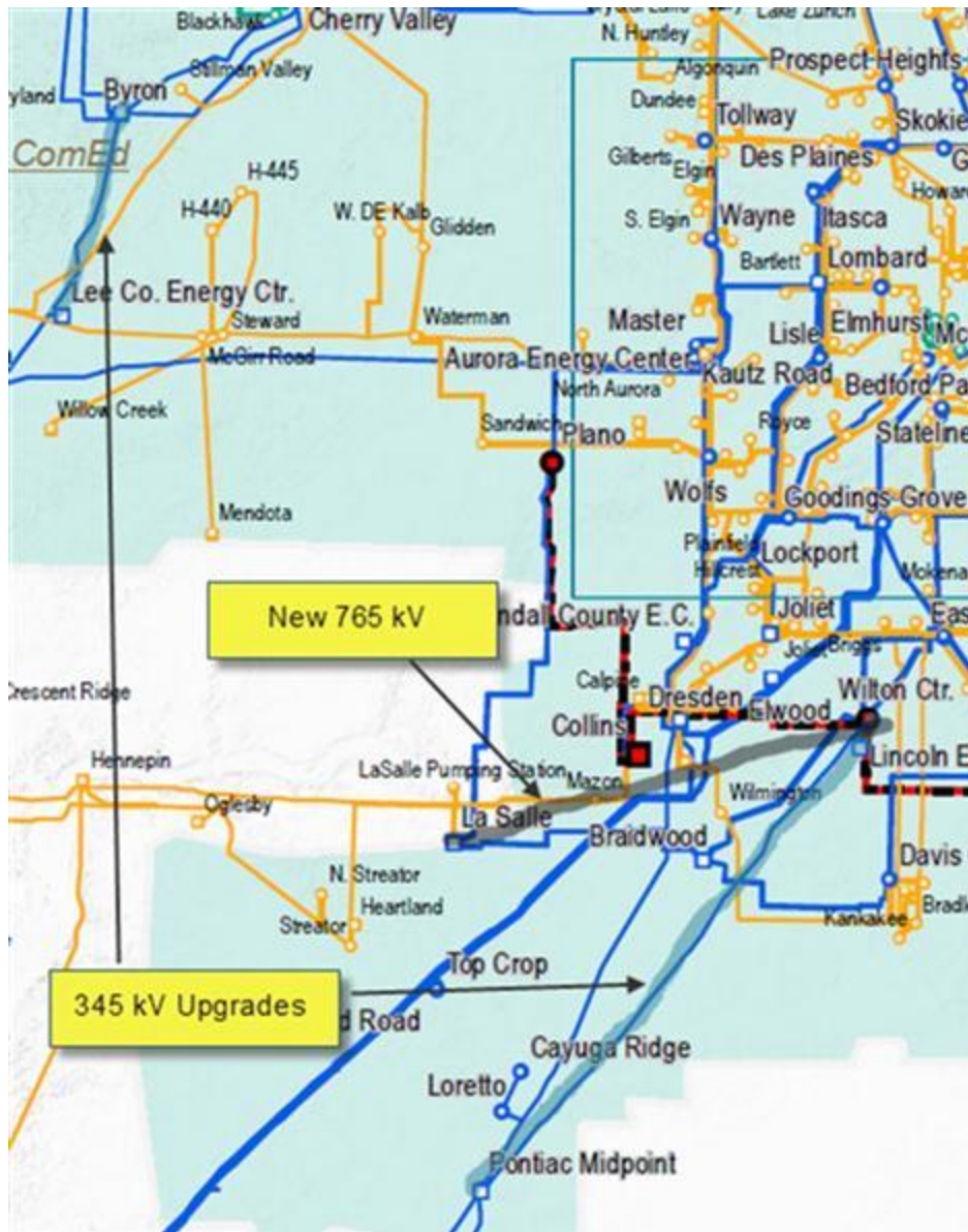
Figure 1-45: 30% HOBO Transmission Overlay – ComEd
