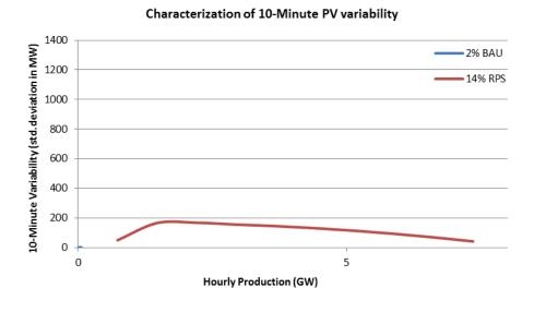
Figure 1-78: Characterization of 10-Minute PV Variability for Lower Penetration Scenarios (Note: 2% BAU 71MW Nameplate Capacity)
