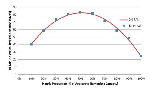
Figure 1-57: Statistical Characterization of 10-Minute Wind Variability for The 2% BAU Scenario
