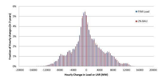
Figure 1-39: Hourly Change in PJM Load and Net Load For 2% BAU Scenario (3 Years of Data)
