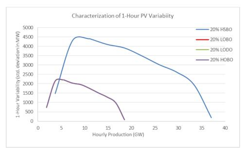
Figure 1-88: Expected 1-Hour Persistence Forecast Error as Function of Current PV Production Level For 20% Scenarios (Note LOBO, LODO and HOBO Scenarios Use Same PV Sites)
