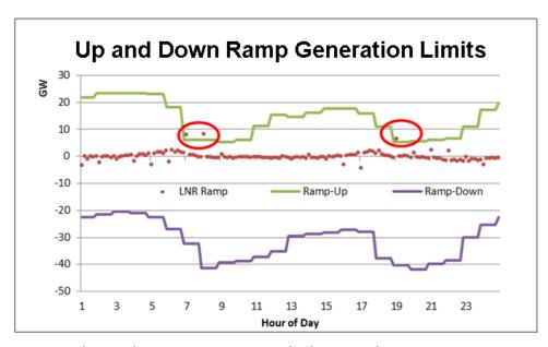
Figure 2-10: Sample Day Showing 10-Minute Periods That Exceed Ramp-Up or Ramp-Down Limits
