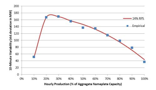
Figure 1-68: Statistical Characterization of 10-Minute PV Variability for The 14% RPS Scenario
