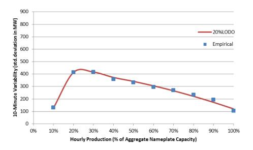
Figure 1-71: Statistical Characterization of 10-Minute PV Variability for The 20% LODO Scenario
