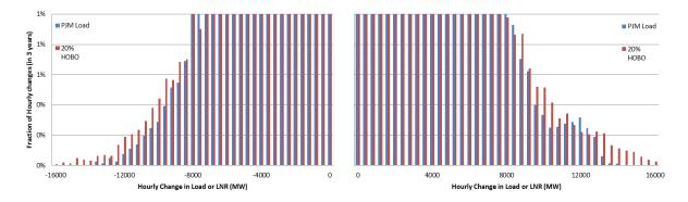
Figure 1-45: Distribution Tails of Hourly Changes for PJM Load and Net Load for 20% HOBO Scenario
