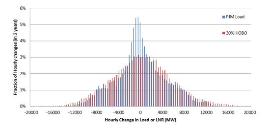
Figure 1-43: Hourly Change in PJM Load and Net Load For 30% HOBO Scenario (3 Years of Data)
