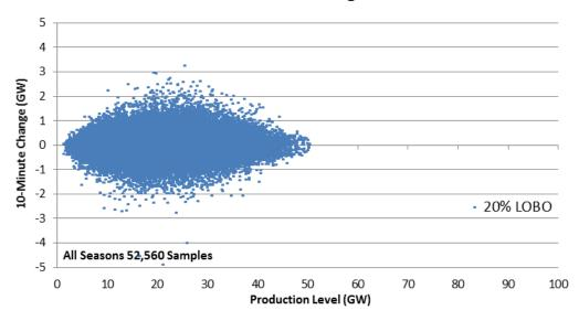
Figure 1-51: 10-Minute Wind + Solar Variability as a Function of Production Level For 20% LOBO Scenario
