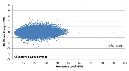
Figure 1-49: 10-Minute Wind + Solar Variability as a Function of Production Level For 20% HOBO Scenario
