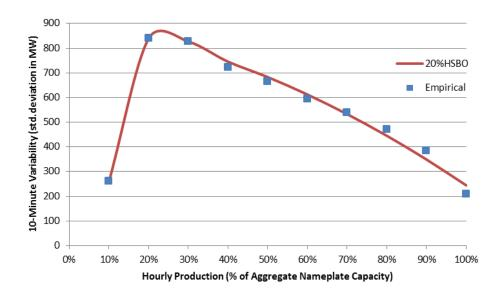
Figure 1-69: Statistical Characterization of 10-Minute PV Variability for The 20% HSBO Scenario
