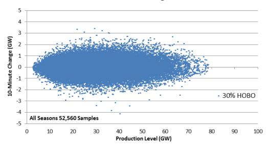
Figure 1-53: 10-Minute Wind + Solar Variability as a Function of Production Level For 30% HOBO Scenario
