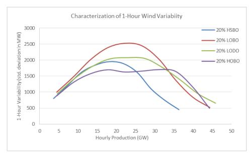
Figure 1-87: Expected 1-Hour Persistence Forecast Error as Function of Current Wind Production Level For 20% Scenarios
