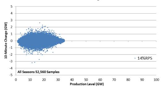
Figure 1-48: 10-Minute Wind + Solar Variability as a Function of Production Level For 14% RPS Scenario
