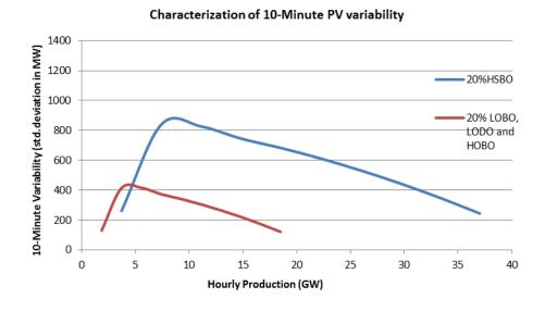
Figure 1-80: Characterization of 10-Minute PV Variability For 20% Penetration Scenarios (LOBO, LODO and HOBO Have Identical PV Sites)
