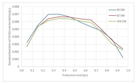
Figure 2-8: 10-Minute Variability of Illustrative Wind Scenarios with Hourly Average Production Level: Empirical Data, Per-Unit of Aggregate Nameplate Capacity for Each Scenario
