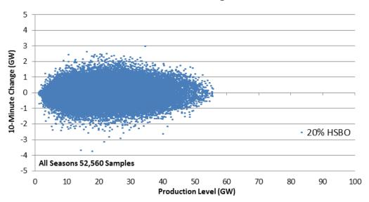
Figure 1-52: 10-Minute Wind + Solar Variability as a Function of Production Level For 20% HSBO Scenario
