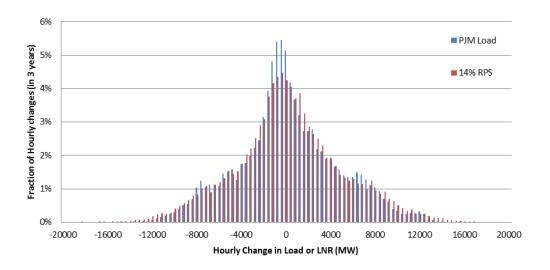
Figure 1-40: Hourly Change in PJM Load and Net Load For 14% RPS Scenario (3 Years of Data)
