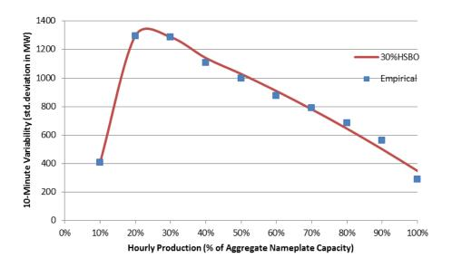
Figure 1-73: Statistical Characterization of 10-Minute PV Variability for The 30% HSBO Scenario
