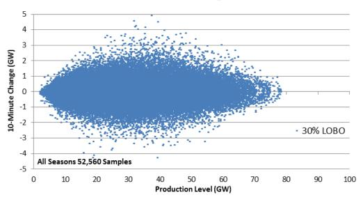
Figure 1-55: 10-Minute Wind + Solar Variability as a Function of Production Level For 30% LOBO Scenario
