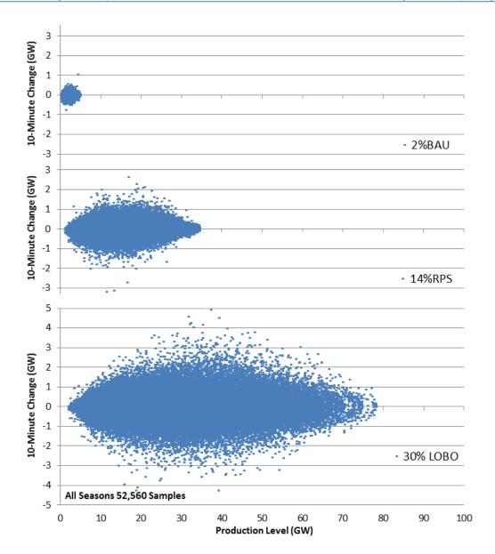
Figure 2-6: 10-Minute Wind and Solar Variability as Function of Production Level for 2% BAU, 14% RPS, and 30% LOBO Scenarios
