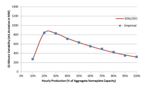
Figure 1-75: Statistical Characterization of 10-Minute PV Variability for The 30% LODO Scenario
