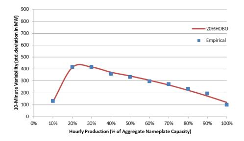
Figure 1-72: Statistical Characterization of 10-Minute PV Variability for The 20% HOBO Scenario
