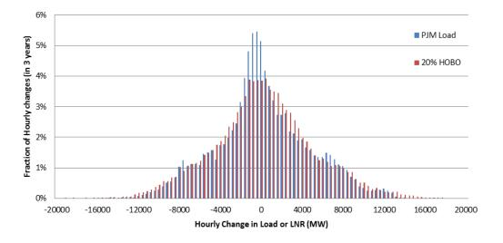
Figure 1-41: Hourly Change in PJM Load and Net Load For 20% HOBO Scenario (3 Years of Data)
