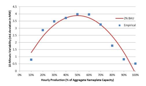
Figure 1-67: Statistical Characterization of 10-Minute PV Variability for The 2% BAU Scenario
