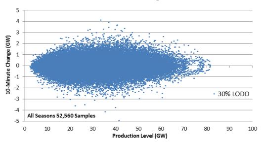
Figure 1-54: 10-Minute Wind + Solar Variability as a Function of Production Level For 30% LODO Scenario
