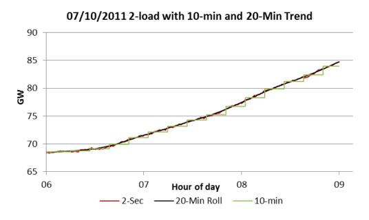
Figure 2-3: 2-Second Load Data Plotted with 20-Minute Rolling Average and 10-Minute Average Load
