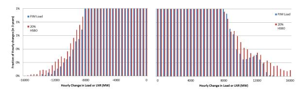
Figure 1-46: Distribution Tails of Hourly Changes for PJM Load and Net Load for 20% HSBO Scenario
