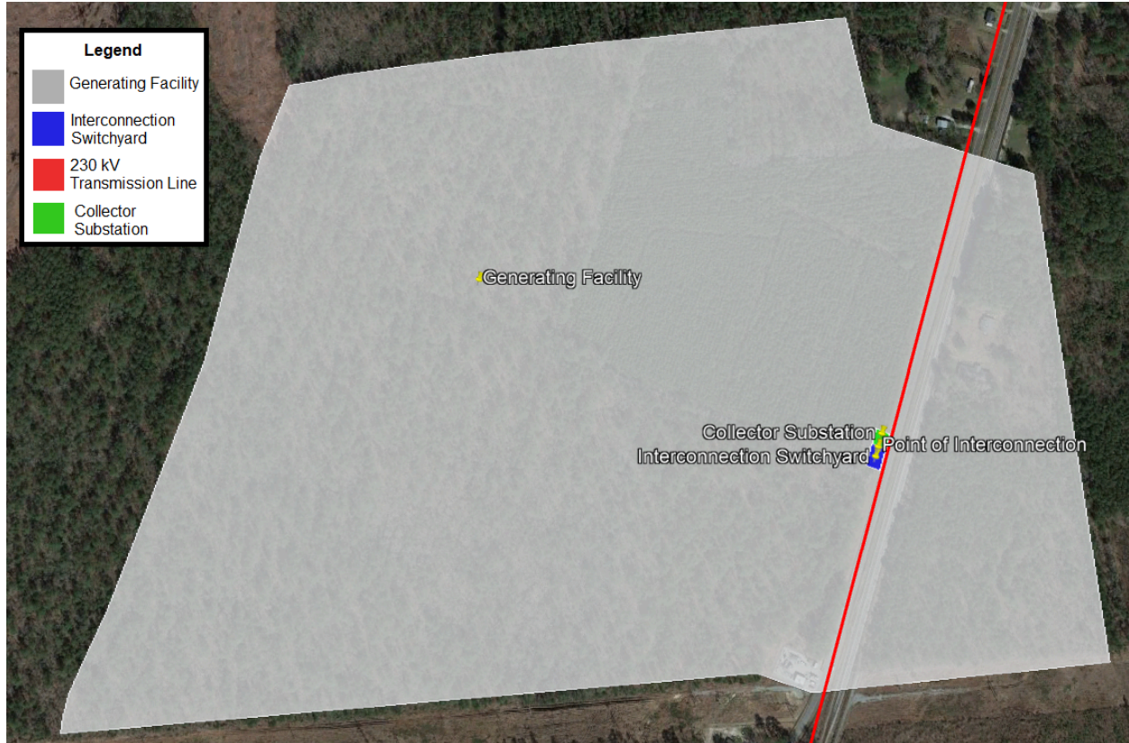
Exhibit 46: Tapping an Existing Transmission Line
