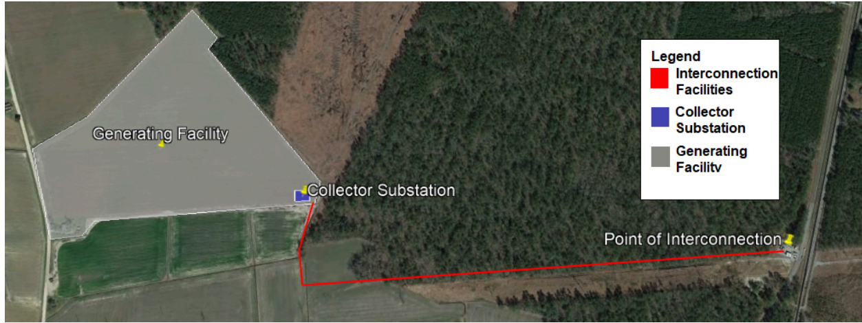
Exhibit 45: Interconnecting into an Existing Substation
