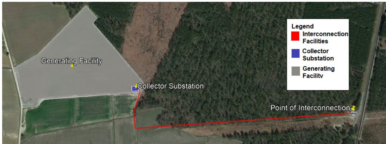
Exhibit xx: Interconnecting into an Existing Substation.
