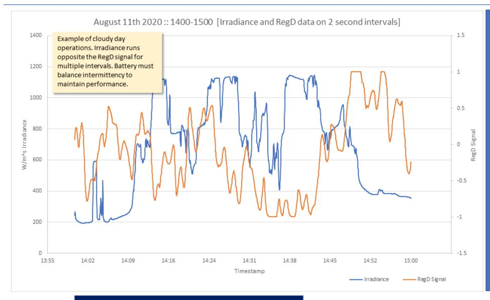
The chart demonstrates the asymmetry that would exist between solar and battery units part of a hybrid resource.
