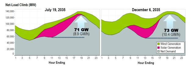
Figure 17. Total Climb From Beginning to End of the Ramping Period for Selected Summer and Winter Days
