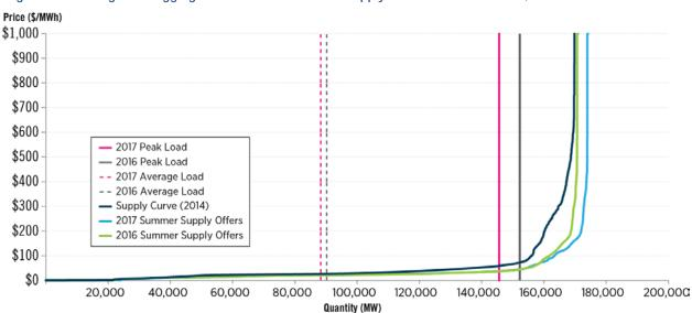
Figure 2. Average PJM Aggregate Real-Time Generation Supply Curves in Summer 2014, 2016 and 2017
