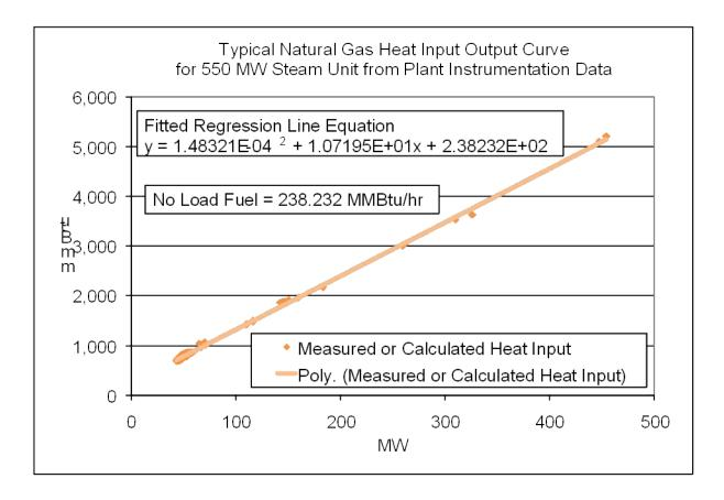
Each diamond in the graph above indicates one hourly heat input data point calculated from plant instrumentation during operations. A regression analysis was performed on the data collected to obtain the unit's Heat Input curve as a function of various unit output levels with oil as a fuel:
