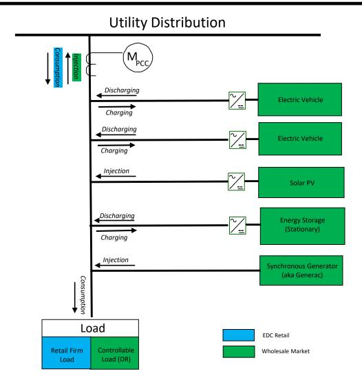
This diagram does not illustrate all customer connection requirements (i.e. disconnect switches)
