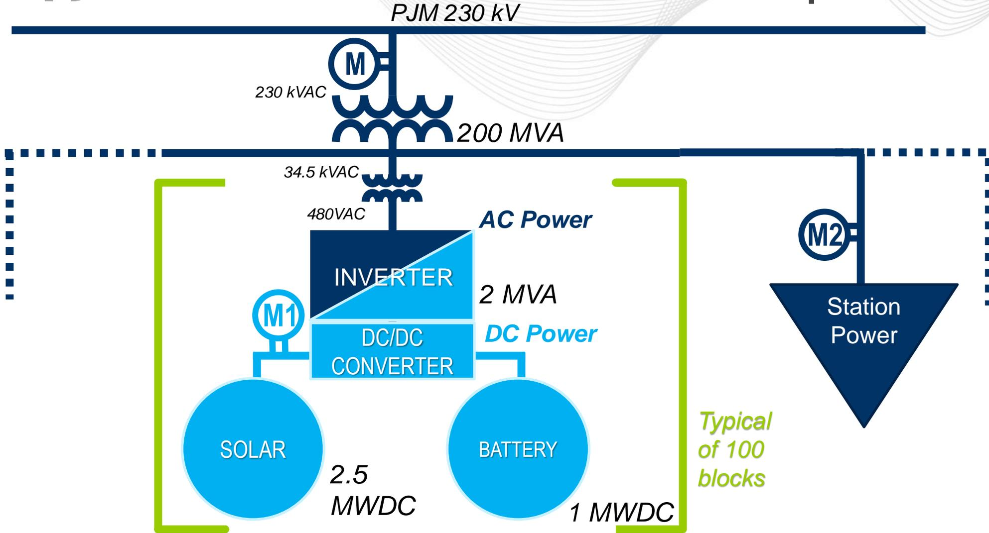
*Example of inverter-based DC-coupled solar-storage hybrid*
