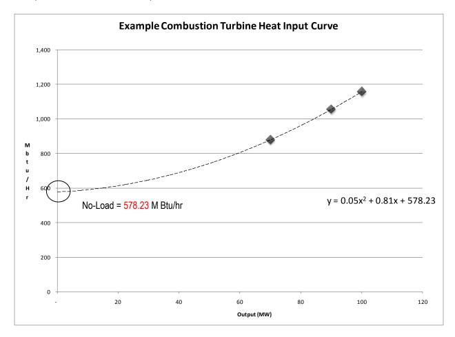
The table below shows the input in MBTU/hour, output in MW, heat rate at different levels of output and incremental heat rate. This test was done at 59 degrees, and since heat rates can change with temperature for most combustion turbines, this temperature is noted so that the reader understands that this may not be the heat rate curve or no-load levels in every 5/11
