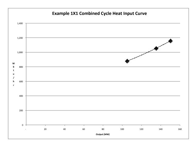
The table below shows the input in MBTU/hour, output in MW, heat rate at different levels of output and incremental heat rate. This test was done at 59 degrees, and since heat rates can change with temperature. These numbers correspond to what is shown in the points in the graph above.
