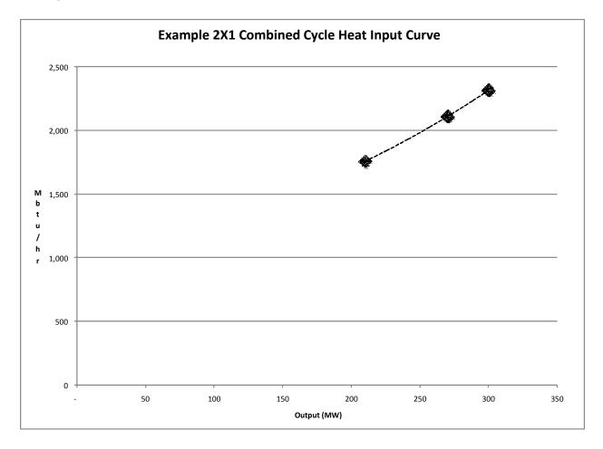
The table below shows the input in MBTU/hour, output in MW, heat rate at different levels of output and incremental heat rate. These numbers correspond to what is shown in the points in the graph above.
