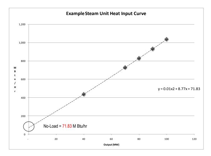
The table below shows the input in MBTU/hour, output in MW, heat rate at different levels of output and incremental heat rate. These numbers correspond to what is shown in the graph above. The red 71.83 MBTU/hour is the no-load fuel, which when multiplied by the fuel costs gives us the no-load cost for the cost based offer.
