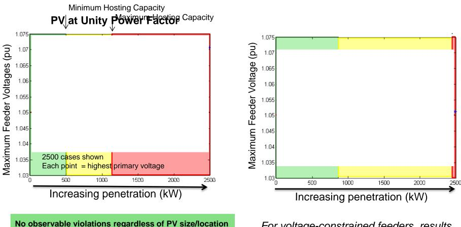
For voltage-constrained feeders, results indicate use of smart inverters can increase feeder hosting capacity for PV
