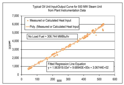
Each diamond in the graph above indicates one hourly heat input data point calculated from plant instrumentation during operations. A regression analysis was performed on the data collected to obtain the unit's Heat Input curve as a function of unit's output with oil as a fuel:
