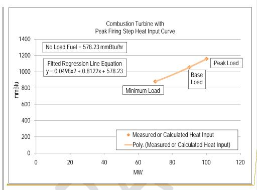
Each marker in the graph above is a design heat input data point obtained from the original equipment manufacturer or calculated by heat balance. A regression analysis can be performed on the design data to obtain the unit's Heat Input curve as a function of Output with natural gas as a fuel:
