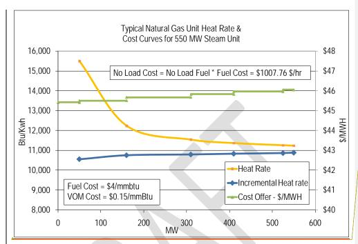
To avoid making adjustments to the No-Load, first calculate the unit's Incremental Cost (\$/MWh) at various outputs using the derivative of the Heat Input Curve:
