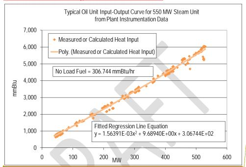
Each marker in the graph above indicates one hourly heat input data point calculated from plant instrumentation during operations. A regression analysis was performed on the data collected to obtain the unit's Heat Input curve as a function of Output with oil as a fuel:
