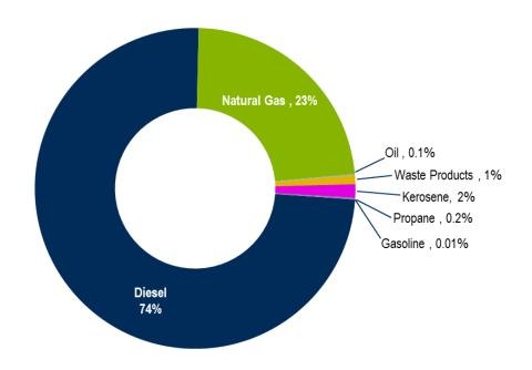
Fuel mix for behind the meter generation that participates in Capacity Market as Demand Response for DY 2016/17 predominantly consists of diesel (74%) and natural gas (23%) which make up a combined 97% of the total fuel types.
