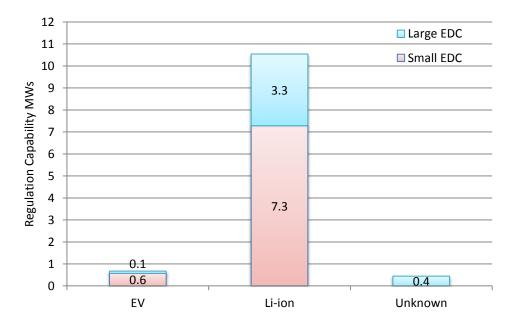
Figure 12: DR DER Registered Regulation Capability from Batteries by EDC size by Technology
