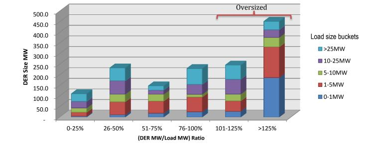
Figure 6: DR DER Registered MW Capability (16/17 DY) by Size and ratio of Size/Load
