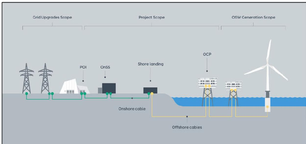
*Note: OCP is interlink-capable. Interlinks offer the ability to connect to other OCPs (not shown)*
