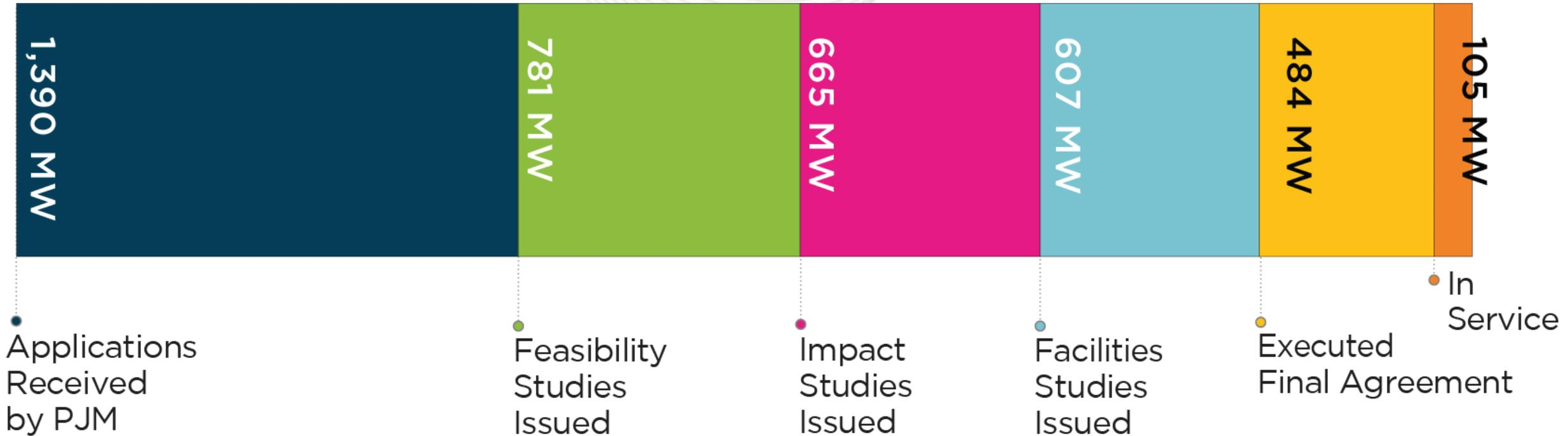
Following Final Agreement execution, 50 MW of capacity withdrew from PJM's interconnection process. Another 329 MW have executed agreements but were not in service as of December 31, 2016. Overall, 7% of requested capacity MW reaches commercial operation. The PJM average is 11%.
