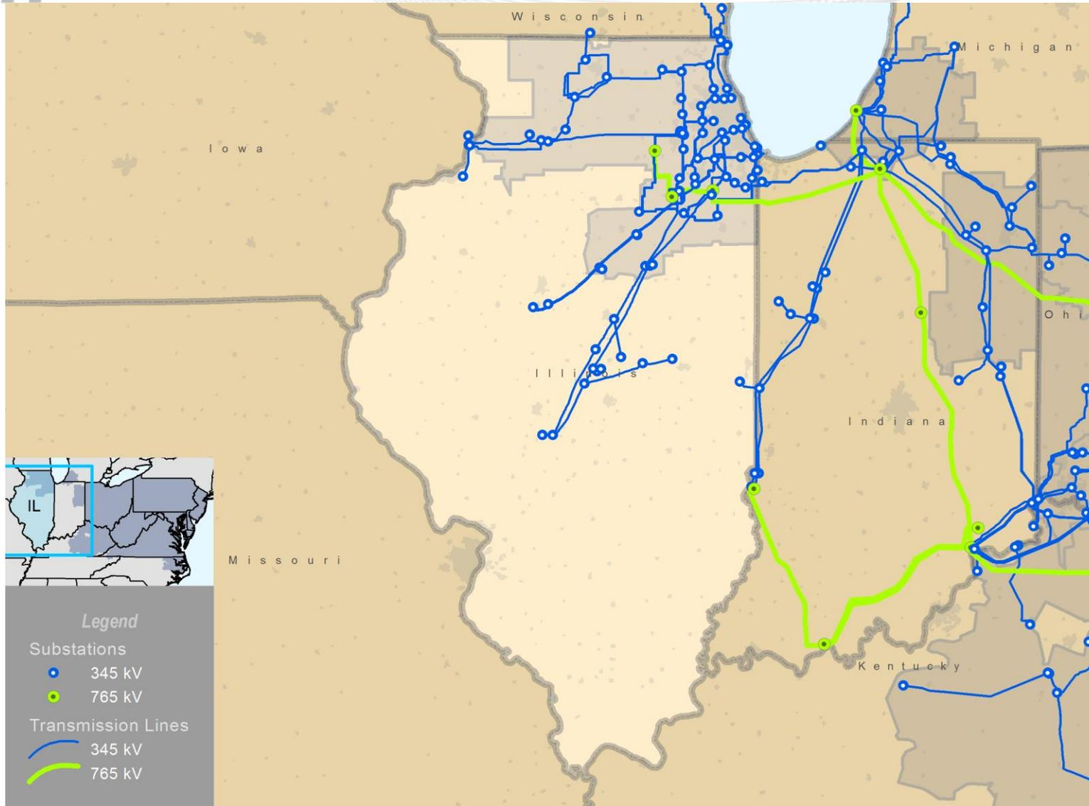
PJM operates the bulk electric system facilities (and others monitored at lower voltages), in northern Illinois. This map includes those of Commonwealth Edison (ComEd). Northern Illinois's transmission system delivers power to customers from native generation resources and those throughout the RTO – arising out of PJM market operations – as well as power imported interregionally from systems outside PJM.
