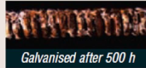
Salt spray test (ASTM B 117, DIN SS 50021)
