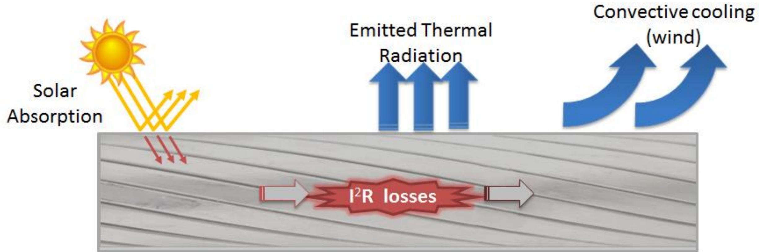
IEEE 738 methodology calculates ampacity based on conductor properties and environmental assumptions:
