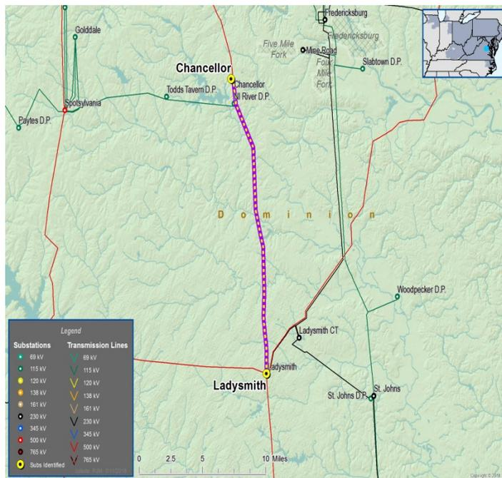
The recommended solution to address the Bristers to Chancellor 500 kV End of Life TO Criteria violation is to rebuild the 500 kV line (21.6 miles), increasing the ampacity from 3,364 to 5,000 amps. This rebuild will utilize the standard single circuit 500 kV tower design. The estimated cost for this work is \$64.65 million, and the required in-service date is immediate. The local transmission owner, Dominion, will be designated to complete this work.
