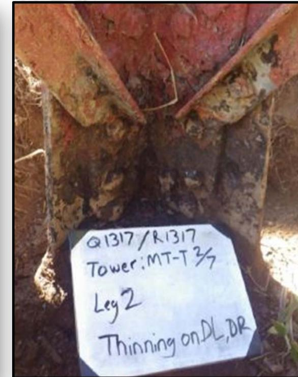
Figure 1: Examples of 25-30% foundation structure loss
