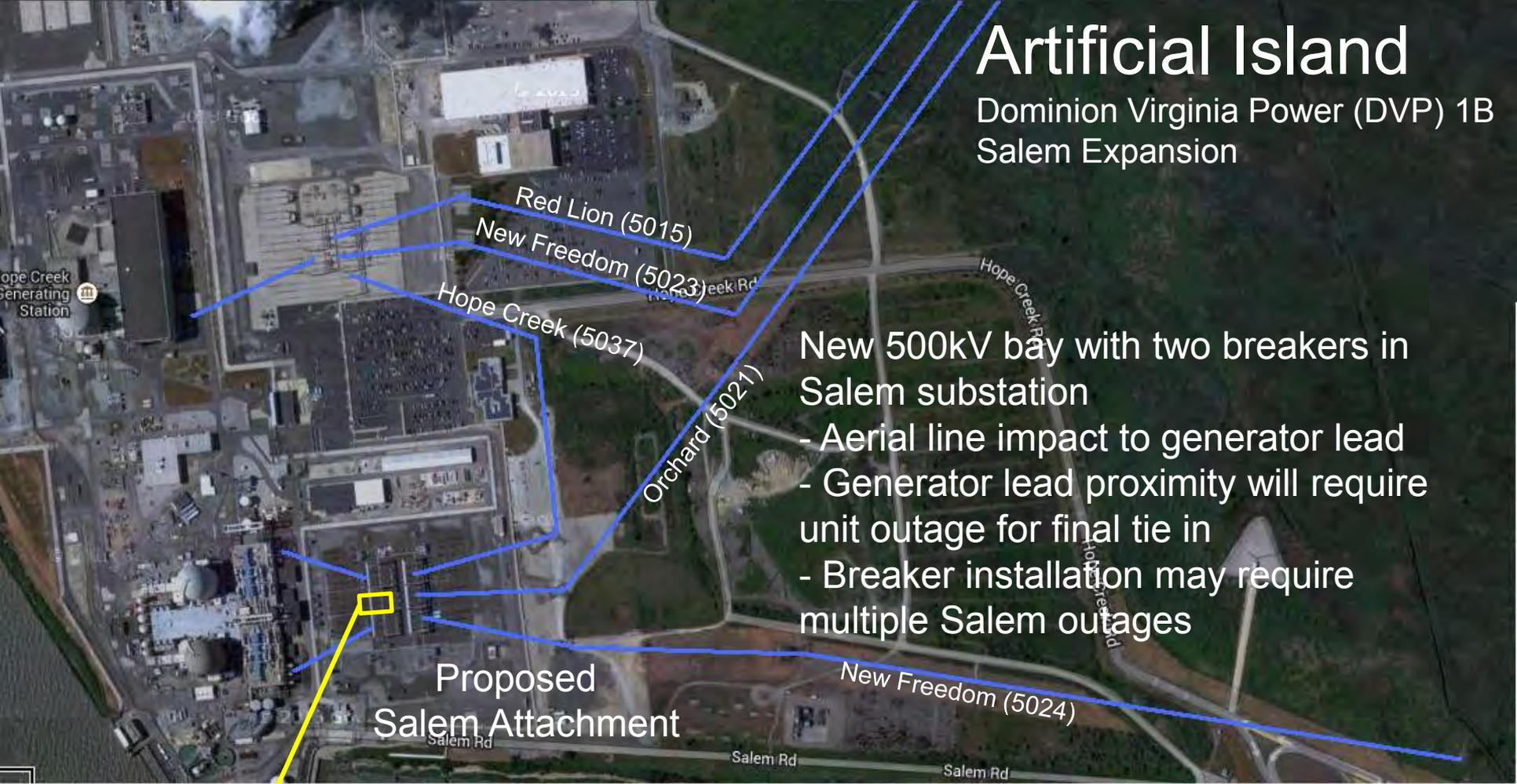
New 500kV bay with two breakers in Salem substation
