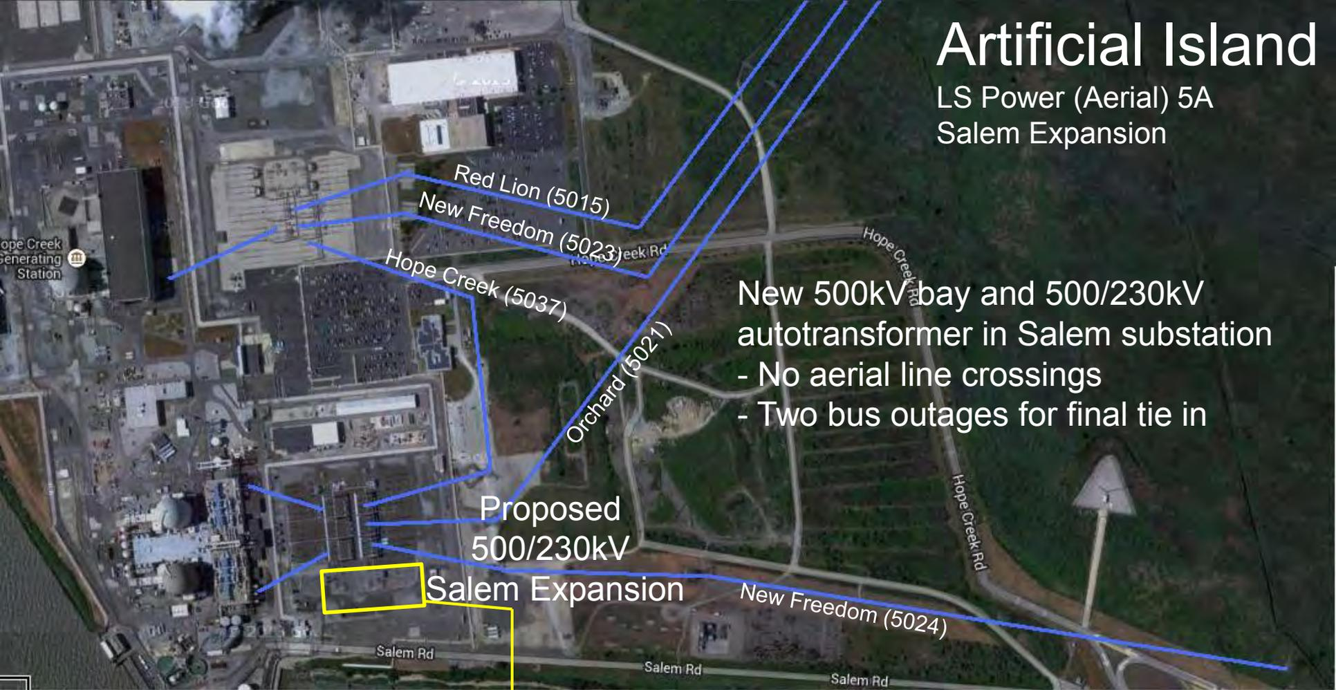
New 500kV bay and 500/230kV autotransformer in Salem substation
