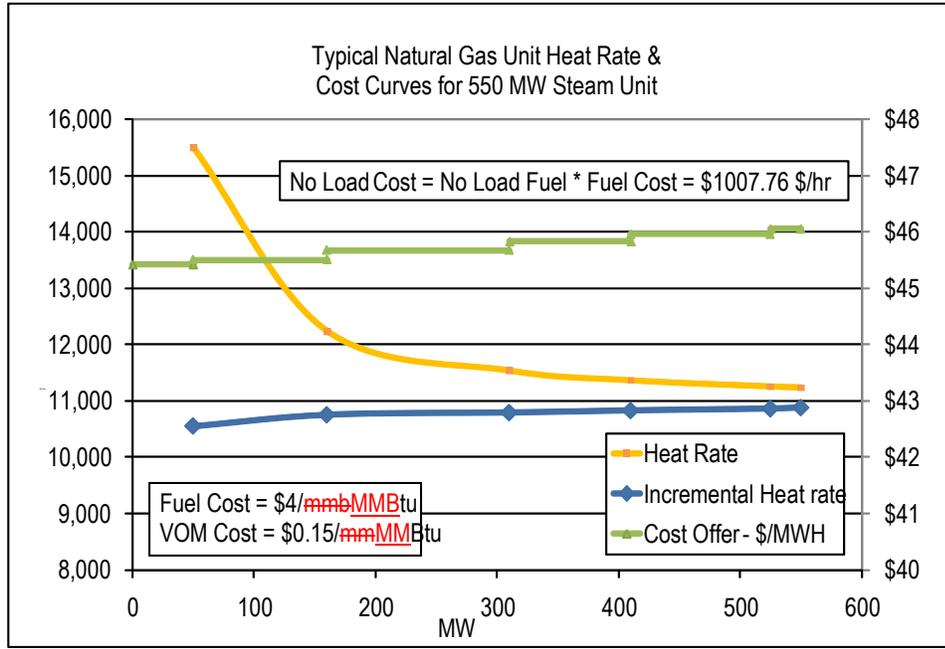
To avoid making adjustments to the No-Load ~~eCost~~, first calculate the unit's Incremental Cost (\$/MWh) at various outputs using the derivative of the Heat Input Curve:
