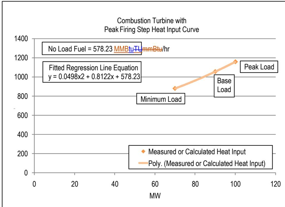
Each diamond in the graph above is a design heat input data point obtained from the original equipment manufacturer or calculated by heat balance. A regression analysis was performed on the design data to obtain the unit's Heat Input curve as a function of unit's oOutput with natural gas as a fuel:
