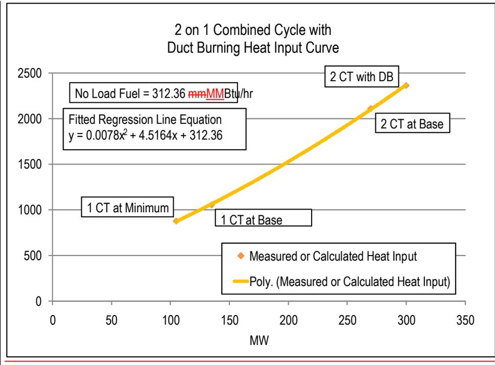
Each diamond in the graph above is a design heat input data point obtained from the original equipment manufacturer or calculated by heat balance. A regression analysis was performed on the design data to obtain the unit's Heat Input curve as a function of unit oOutput levels with natural gas as a fuel:
