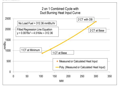
Each diamond in the graph above is a design heat input data point obtained from the original equipment manufacturer or calculated by heat balance. A regression analysis was performed on the design data to obtain the unit's Heat Input curve as a function of <u>unit o</u>Output <u>levels</u> with natural gas as a fuel:
