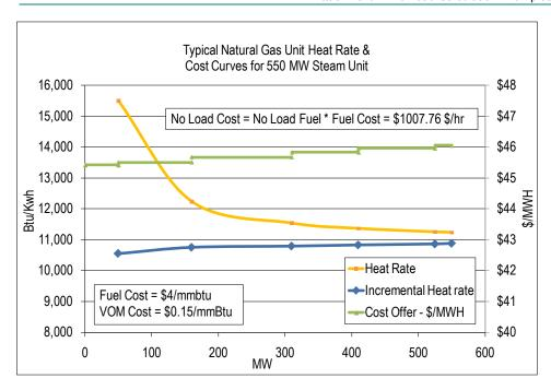
To avoid making adjustments to the No-<u>IL</u>oad <u>cost</u>, first calculate the unit's Incremental Cost (\$/MWh) at various outputs using the derivative of the Heat Input Curve:
