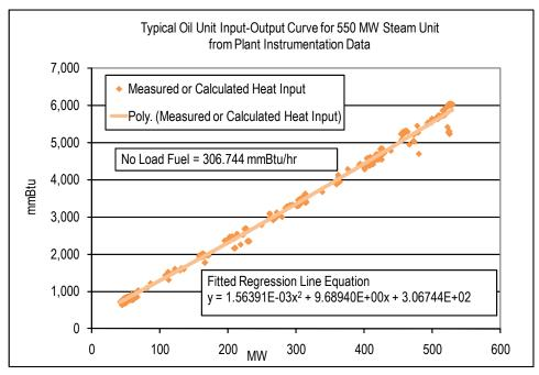
Each diamond in the graph above indicates one hourly heat input data point calculated from plant instrumentation during operations. A regression analysis was performed on the data collected to obtain the unit's Heat Input curve as a function of <a href="mailto:unit's ocupation">unit's ocupation</a> ocupation with oil as a fuel:
