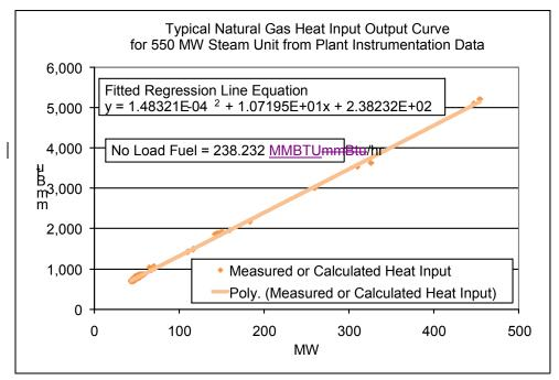
Each diamond in the graph above indicates one hourly heat input data point calculated from plant instrumentation during operations. A regression analysis was performed on the data collected to obtain the unit's Heat Input curve as a function of <a href="mailto:various unit o@utput\_levels">various unit o@utput\_levels</a> with oil as a fuel:
