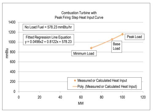
Each diamond in the graph above is a design heat input data point obtained from the original equipment manufacturer or calculated by heat balance. A regression analysis can be performed on the design data to obtain the unit's Heat Input curve as a function of <a href="mailto:various unit o@utput\_levels">various unit o@utput\_levels</a> with natural gas as a fuel:
