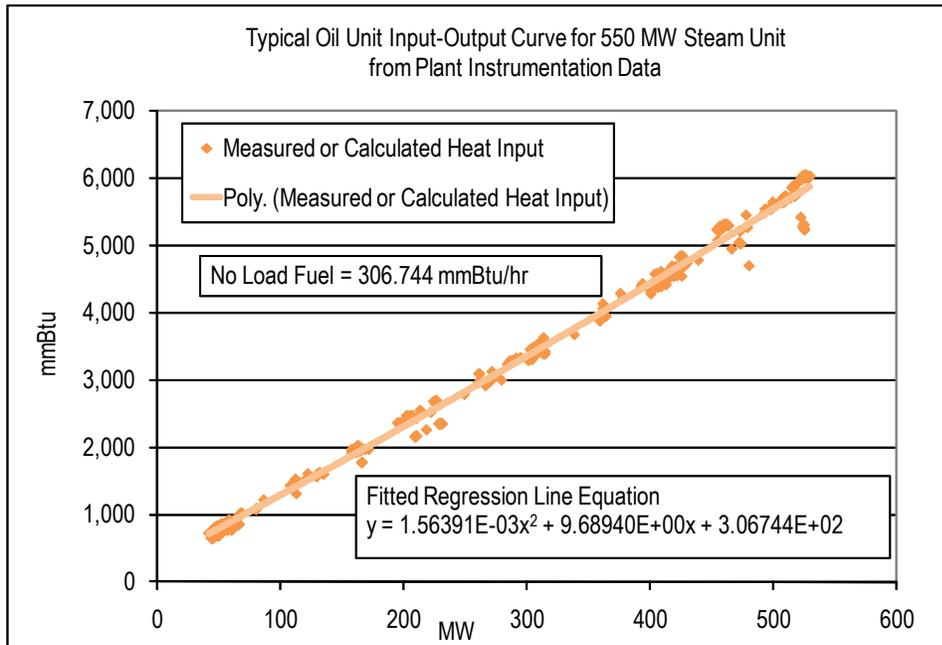
Each diamond in the graph above indicates one hourly heat input data point calculated from plant instrumentation during operations. A regression analysis was performed on the data collected to obtain the unit's Heat Input curve as a function of unit's Output with oil as a fuel:
