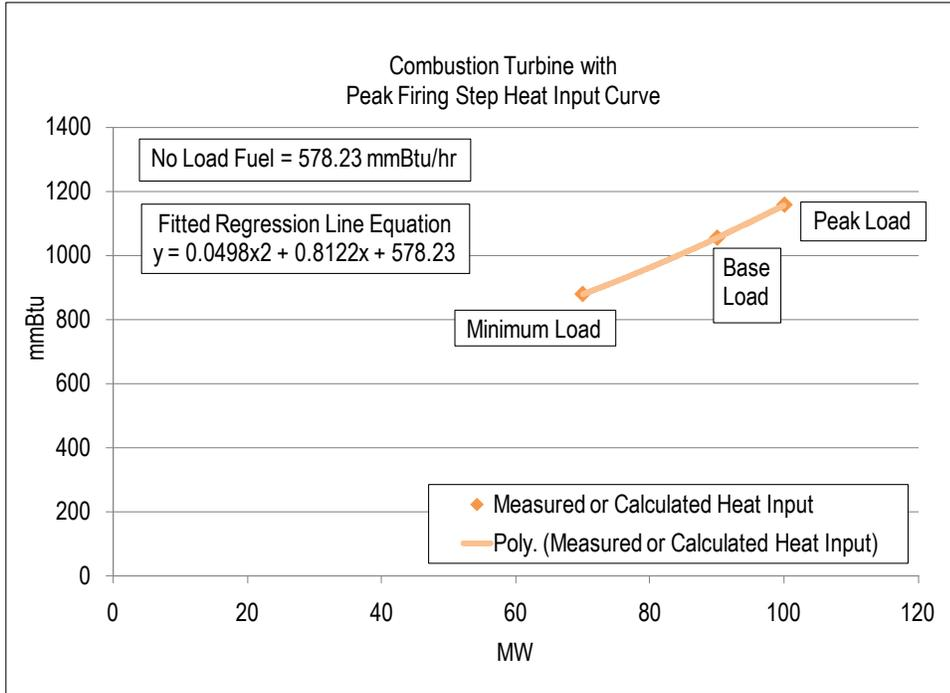
Each diamond in the graph above is a design heat input data point obtained from the original equipment manufacturer or calculated by heat balance. A regression analysis can be performed on the design data to obtain the unit's Heat Input curve as a function of various unit oOutput levels with natural gas as a fuel:
